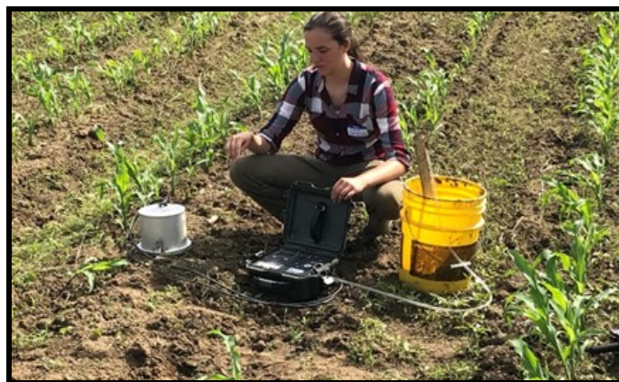
Stella Pey demonstrating the water infiltration rate test
