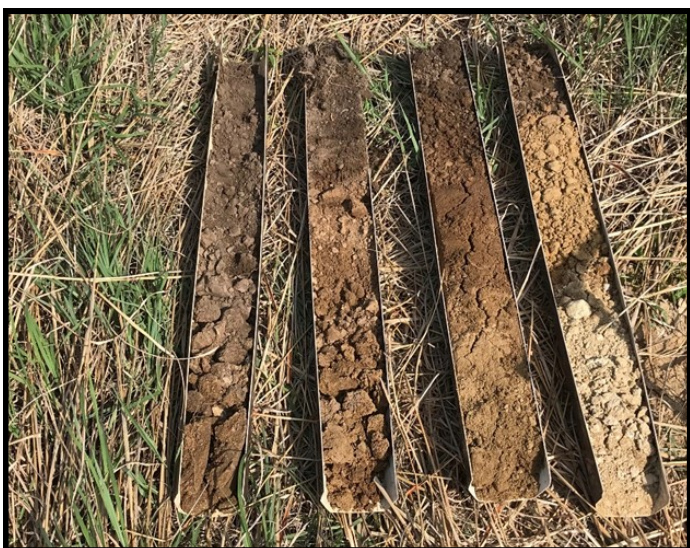
Far Left – Undisturbed fence line – 24 inches of A horizon topsoil 2 nd from left – 30 years of CRP – 14 inches of A horizon topsoil 3 rd from left – 5 years of CRP – Nearly 10 inches of A horizon topsoil Far right – continuous row-crop – 8 inches of A horizon topsoil
